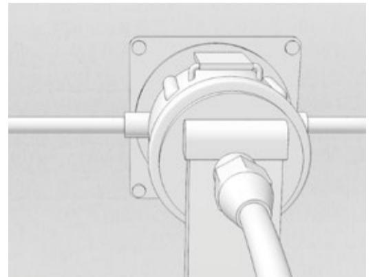
Connect coupling into corresponding cleaning socket.
