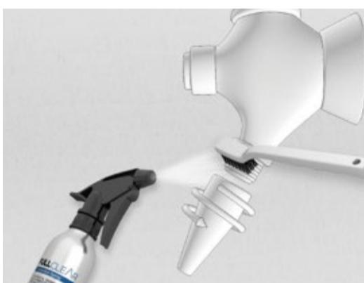
Remove nozzles / sparklers. Spray and clean threads using the brush provided, then spray again once clear of all contaminants.
