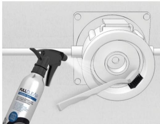
Spray around the cleaning sockets removing all visible contaminants using the brush provided and re-spray.
