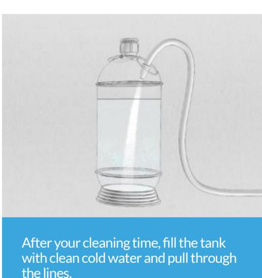
After your cleaning time, fill the tank with clean cold water and pull through the lines.
