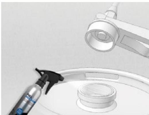
Disconnect keg couplings and spray each part using the FullClear Connector Spray provided.
